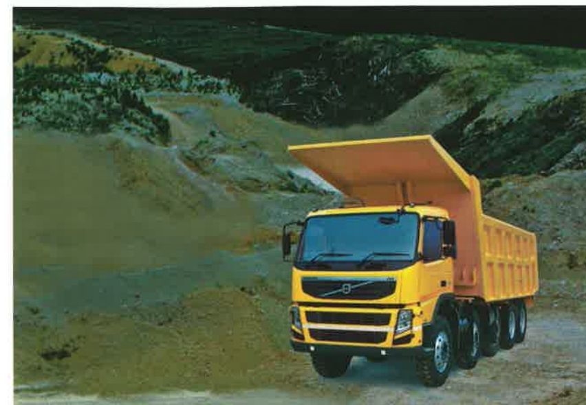
Volvo FM 480 10x4 dump truck comes with 24 M3 rock body.
