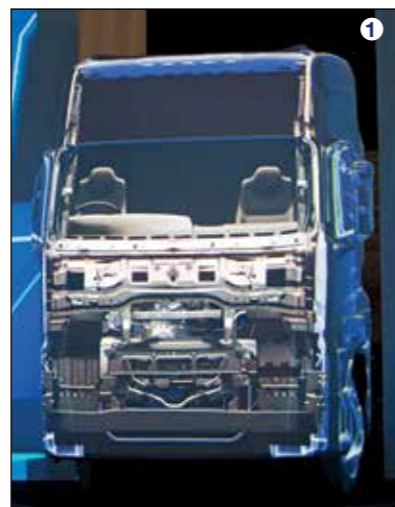
2. The Pro 8049, a 49 tonne GVW, 6x4 tractor powered by a 280HP engine is the flagship product of the range.
